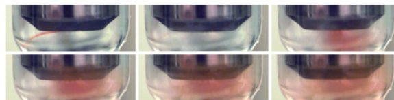
Figure 2. Mixing pattern of solution (red, flowing from the tapped ultrasonic horn) and antisolvent (white, flowing from the lower right) within the spray sonocrystallization rig. The second frame marks the start of sonication. Frames were extracted from video every 33 ms.
