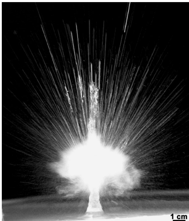
Figure 13. Photograph of an ultrasonic fountain and mist produced at 1.7 MHz. Reproduced with permission from [191]. Copyright 2005, American Chemical Society.
